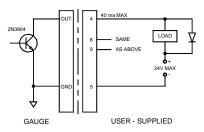
results of the comparisons are indicated through the three open-collector outputs provided on the 9-pin connector, thus providing "under", "in range" and "over" signaling. These outputs can be connected to indicators, buzzers or relays as required for the application.
