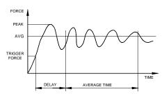
mable parameters associated with this mode: trigger force, initial delay and average time. The programming of these parameters and the enabling of the Average mode are done during the gauge setup. Please refer to the "Configuration" section for more information
